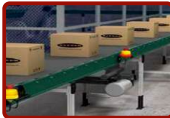
Stop Buttons on a Conveyor
