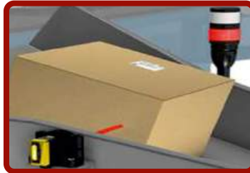
Jam Indication on a Conveyor
